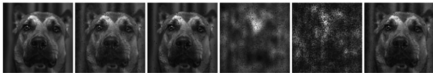
Fig. 8 Results for dog dataset with the binary mask. From left to right: ground truth, Fienup (PSNR, 28.40 dB; SSIM, 0.87), TWF (PSNR, 30.42 dB; SSIM, 0.93), WF (PSNR, 16.89 dB; SSIM, 0.30), PRred (PSNR, 13.55 dB; SSIM, 0.16), proposed (PSNR, 28.88 dB; SSIM, 0.88)
